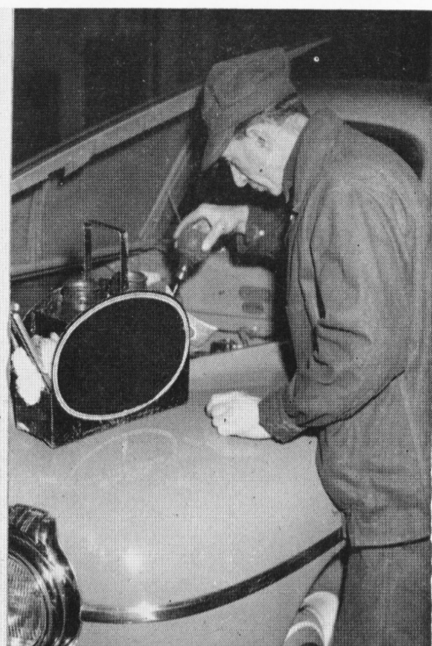
With winter just around the corner, batteries need special consideration. At Scovill they get proper and regular attention. Water and the amount of charge is constantly checked.
