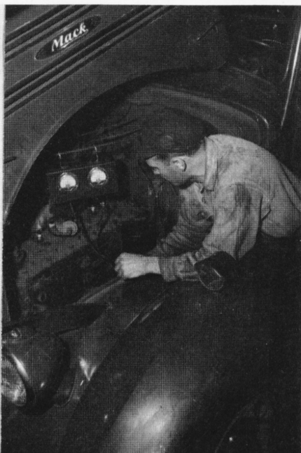
John Vito, tune-up man and night supervisor, is testing the electrical system of a Scovill truck. John is checking up on the generator. He makes minor repairs at night.
