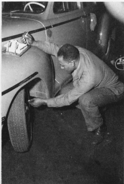
Tire Conservation is an A-1 consideration at the Main Plant. Milton Wyrick tests the air pressure in a tire, using a Schrader gauge. He jots down the readings on a chart.
