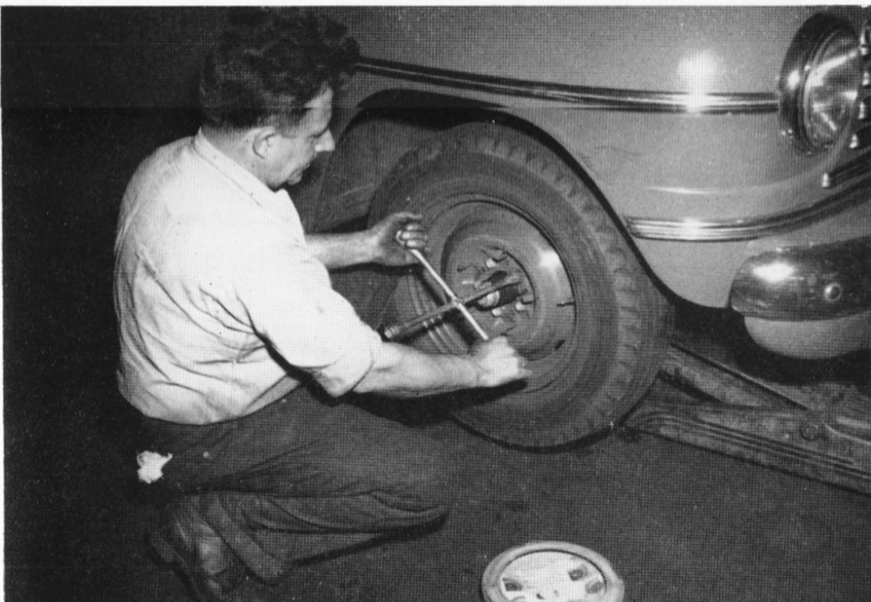
In line with the national tire conservation program — and we are an old hand at conservation — Scovill Transportation Department follows through on all advice for making rubber stretch to the limit. Johnny Sathory removes a tire for recapping before the treads are worn completely away. Tires are changed from wheel to wheel from time to time for even wear.
