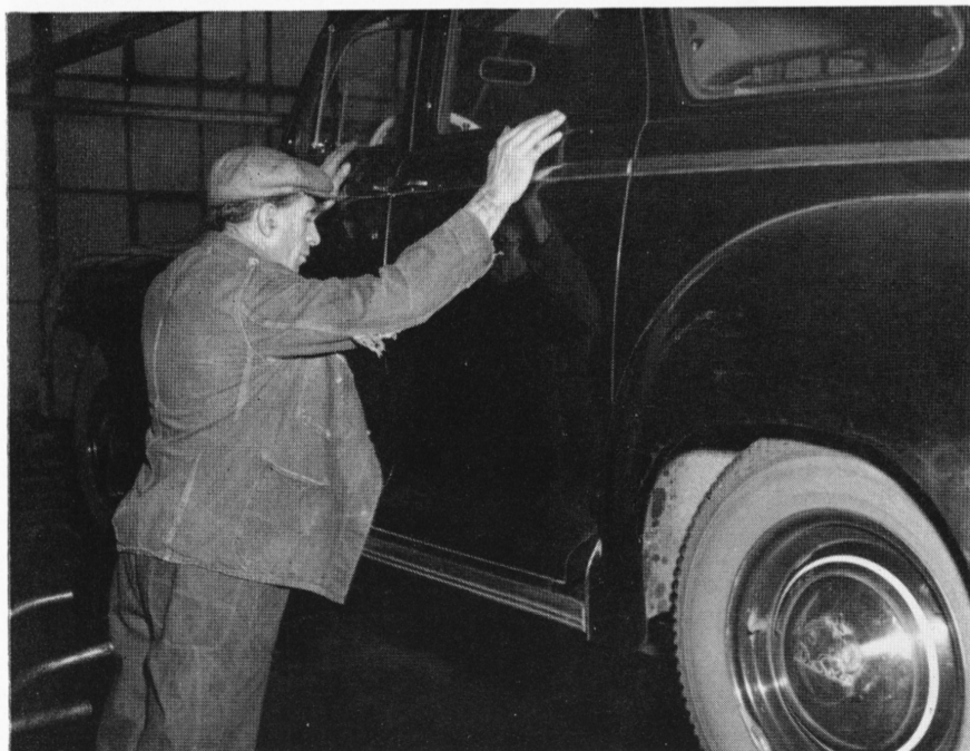
Proper lubrication is a big factor in keeping a car in top running condition. This automobile is being rocked from side to side in order that the mechanic may detect squeaks that indicate friction and the need of grease. Constant attention to the matter of lubrication is given by our mechanics. For that reason our fleet is almost squeak-free.
