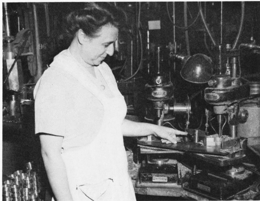
Operators of the high-speed bench drill presses in Chucking are turning out more work with less effort as the result of this idea suggested by Victoria Sacco of the Department. The suggestion has been submitted to the Victory Committee. Victoria points to a rod that leads to an air cylinder under the bench. It operates two presses at once by a press of the foot. Before the device was installed, the operations were done by hand.
