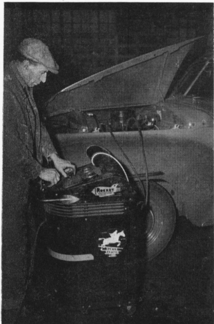
William Woolsey, Garage, charging a battery in a Scovill automobile. It's wise to keep batteries fully charged, in order to insure long life and peak of effectiveness.
